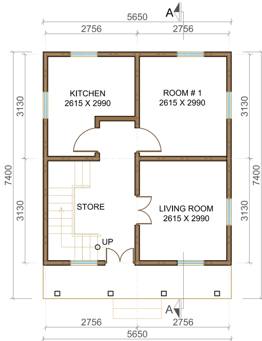
GROUND FLOOR PLAN FLOOR AREA: 36.19 SQ. M.
